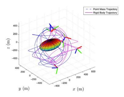
Figure 1. Differences between point mass and rigid body trajectories for a 63 kg spacecraft in proximity to an ellipsoid with mass and size similar to NEA Itokawa (simulated time period is 3700 s).
