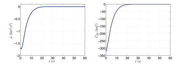
Figure 3. Numerical simulation results showing time evolution of estimation errors for first and one of the second order gravity coefficients of an asteroid the size of Mathilde, obtained from remote measurements by an orbiting spacecraft.
