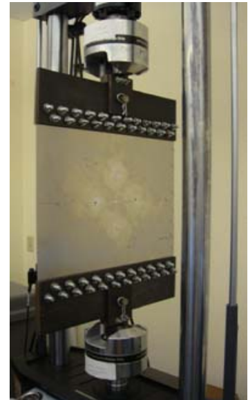
Figure : Plate sample (2-D) mounted in loading jig of MTS load frame for real-time acoustic measurements.
