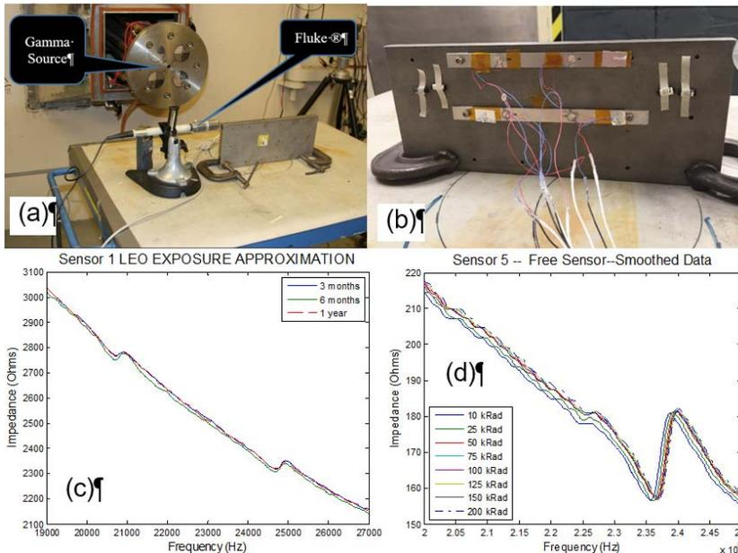
Figure 9 (a) White Sands Co-60 radiation equipment (b) Gamma radiation test setup with free piezoelectric sensors and smart beam structures, (c) structural impedance response at various time equitant to LEO radiation exposure, (d) piezoelectric sensor impedance (in free condition) at various radiation exposures.
