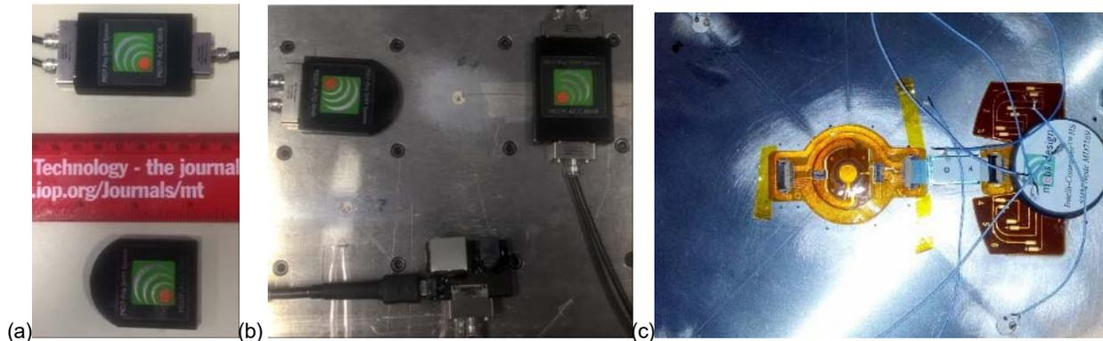
Figure 10 Metis Design hardware for elastic wave propagation and impedance tests: (a) top – Accumulation node and bottom with semicircular cap - signal generation/acquisition node, (b) both nodes are shown along with communication adapter on a realistic satellite panel, (c) older version of hardware flown on an SL8 sub-orbital mission (metisdesign.com).
