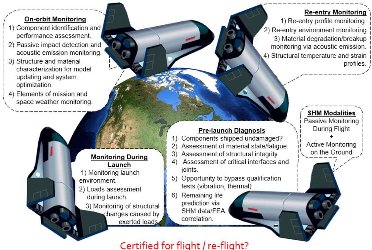
Figure 1 Application of SHM to Reusable Launch Vehicle (RLV). SHM modalities at each stage of spaceflight.
