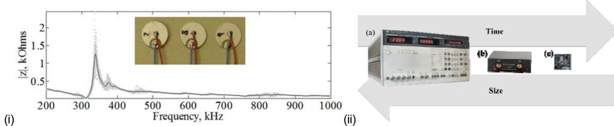
Figure 8 (i) Piezoelectric active SHM sensors (in free condition) and associated impedance spectrum. (ii) Impedance analyzers: (a) HP 4192A, (b) Cypher Instruments C-60, (c) LANL WID3.
