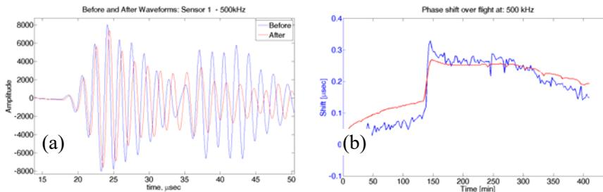
Figure 6 Ultrasonic signals collected during SL8 mission: (a) waveforms acquired before and after the flight, (b) phase shift of the initial pulse vs. time during SL8 mission. Red curve is temperature reading.
