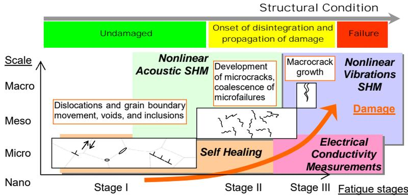
Figure 3 Damage accumulation in a structural system and the SHM methodologies associated with particular damage scales.
