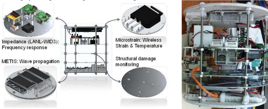
Figure 5 Schematics of payload experiments and a photograph of New Mexico Tech's SL8 payload (during environmental testing) flown on sub-orbital flight November 12, 2013.
