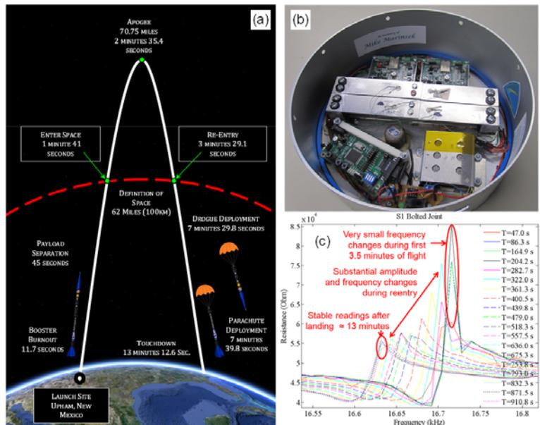
Figure 4 New Mexico Tech SL5 mission: (a) payload trajectory, (b) payload, (c) collected electromechanical impedance data.
