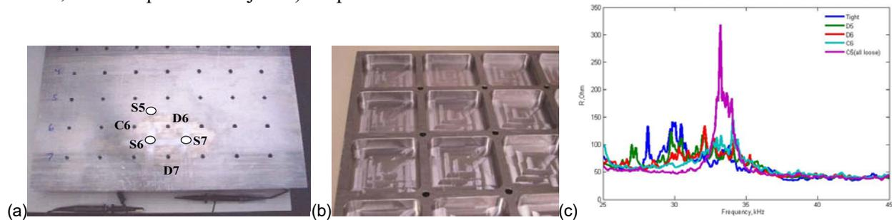
Figure 7 A realistic satellite panel consisting of two aluminum plates with iso-grid frames on the back side: (a) the sensor layout and position of bolts, (b) details of the iso-grid structure, (c) Impedance (real part) changes of sensor S5 as surrounding bolts are loosened incrementally.
